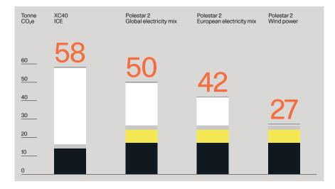
The carbon footprint includes emissions from upstream supplier activities, manufacturing and logistics, use phase of the vehicle and the end-of-life phase. The functional unit chosen is "The use of a specific Polestar vehicle driving 200,000 km".
