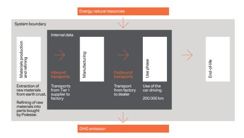
The inventory does not include any processes such as business travel, R&D activities or other indirect emissions. Nor does it include infrastructure e.g. the production and maintenance of buildings, inventories or other equipment used in the production, construction and maintenance of roads or electricity grids. Emissions from tires and road wear is not included in the study. Maintenance of the vehicles is not included in the study due to lack of data.
